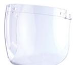
3M™ Faceshield, 5F-11 is our optical class 1, clear curved polycarbonate faceshield with antifog and anti-scratch coating. It's compatible with 3M™ V5 Faceshield System for mounting on 3M™ SecureFit™ X5500 Safety Helmet.
