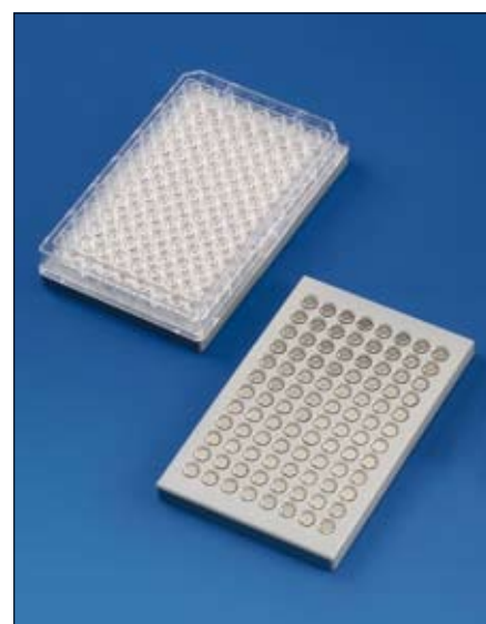
96 Magnet Bar Plate (8 x 12 cm) with 96well culture plate.
