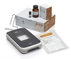
myECL™ Imager for one-touch image capture and analysis of western blots: a powerful and easy-to-use blot and gel documentation instrument for sensitive, multimode image capture and analysis that works with chemiluminescent, colorimetric, or UV light-activated fluorescent substrates or stains.
