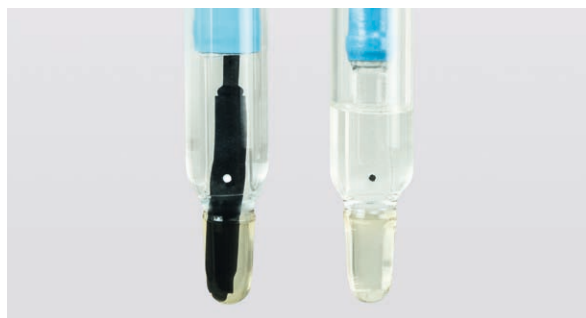
Figure 3: Left to right: clean junction (white "dot") is visible in front of black temperature probe and contaminated junction (black "dot")
