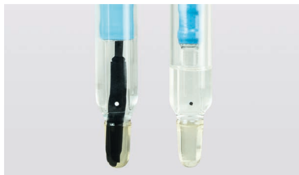
Figure 2: Left to right: clean junction (white "dot") in front of a black temperature probe and contaminated junction (black "dot")
