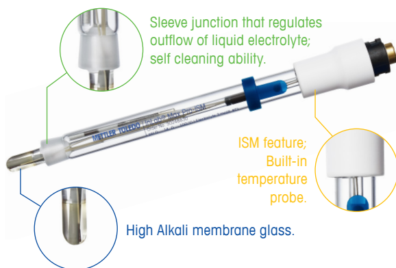
Figure 2: InLab Max Pro-ISM pH sensor.
