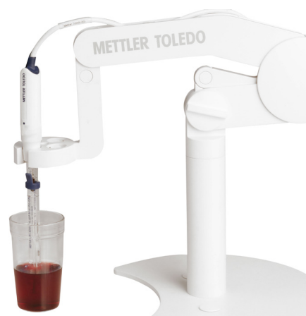
Figure 3: Measuring a wine sample using InLab Max Pro-ISM sensor.
