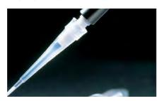
Sample preparation and precise liquid handling in one device. A 0.6µL bed of  $C_{18}$ ,  $C_4$  or SCX (strong cation exchange) media is fixed at the end of a 10µL pipettor tip such that there is no dead volume; concentrated, purified samples are eluted in 1 to 4µL. For applications requiring smaller elution volumes (e.g., <1µL), ZipTip Micro Bed  $C_{18}$  tips feature a microbed format containing 0.2µL of media.
