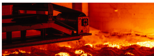
(640A3503) Automated addition of raw material to the DURAN™ glass melting tank
