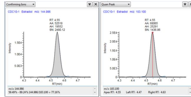
Figure 3. Representative chromatograms of CDC HoSt program samples analyzed here showing both a low and high concentration sample
