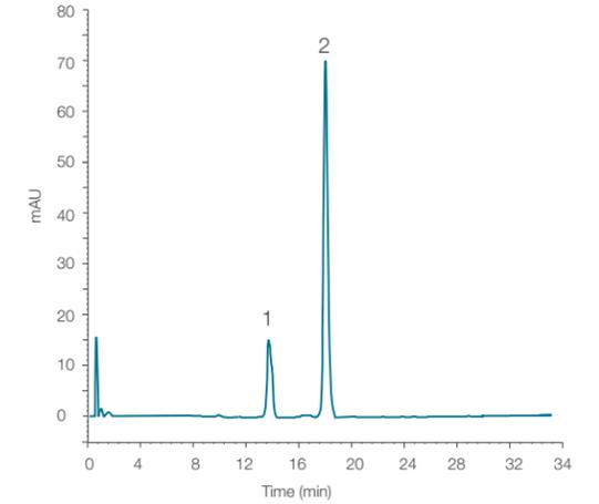
Figure 2. Improved analysis of ibuprofen and valerophenone using a Accucore C18 column
