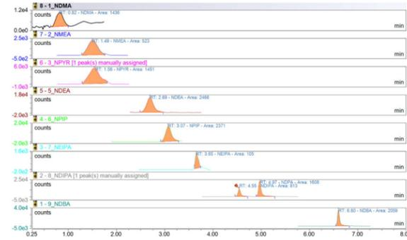
Figure 1. XIC of quantitation ion of nitrosamine impurities in 0.5 ng/mL check standard at a mass tolerance setting of 3 ppm
