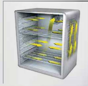
HOMOGENEOUS TEMPERATURE DISTRIBUTION
