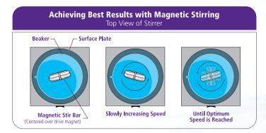
Vertical distance between the drive magnet and the stirring bar should be kept to a minimum for the best coupling and stirring efficiency. Therefore, the containing vessel should be as thin as practical.
