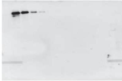
**Fig 4.3.** Comparison of blots following wet and semidry transfer. A two-fold dilution series of transferrin starting at 5  $\mu\text{g}$  was transferred to Amersham™ Hybond P (now replaced by Amersham Hybond P 0.45) membranes (PVDF). Semidry transfer is less efficient for this particular protein than wet transfer; less protein throughout the dilution series is transferred, leading to reduced sensitivity.
