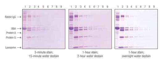
**Figure 35. Enhanced sensitivity and clear background using Imperial Protein Stain.** For even greater sensitivity and reduced background, gels can be stained with Imperial Protein Stain for 1 hour and washed with water from 1 hour to overnight. **Lane 1:** BSA only (6 µg); **Lane 2–9:** loaded left to right with 1,000, 200, 100, 50, 25, 12, 6, and 3 ng protein sample.
