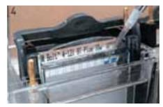
Make sure the wells are completely filled with 1X buffer.
