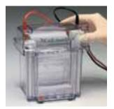
Place the cell lid on the unit and you're ready to run. Figure 26. How to use the XCell SureLock Mini-Cell.
