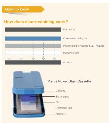
The significant reduction in protein staining time is accomplished by utilizing inonic Power Stain Solution and Destain Solution to electrophoretically drive the negatively charged Coomassie R-250 dye out of the top gel pad, through the polyacrylamide gel matrix and the bottom gel pad, and toward the positively charged anode.
