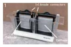
Snap the electrophoresis tank into the base, and place the cassette clamp(s) into the chamber(s) with the anode connector(s) (+) aligned to the center.
