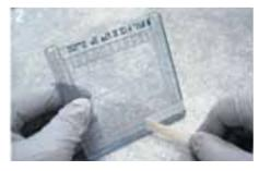
Remove the comb, and peel away the tape at the bottom of the gel cassette.
