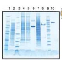
Figure 14. Novex Tricine gel electrophoresis. Protein standards and samples were loaded at 10 µL sample volumes on Invitrogen<sup>™</sup> Novex<sup>™</sup> 10–20% Tricine Protein Gels. Electrophoresis was performed
