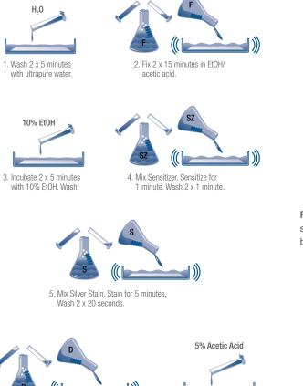
7. Remove developer. Stop with 5% Acetic Acid for 10 minutes.
