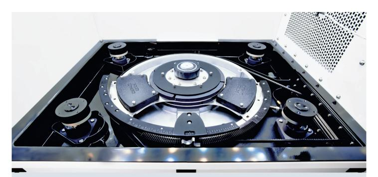
Shake faster, smoother, and longer with the new Eppendorf X-Drive Shaker Mechanism. The five eccentric mounting points for the shaker platform are precisely engineered to ensure long-lasting, repeatable performance for years to come. The four shafts in the corners and Balance Master Technology support precise vibration-free shaking on every point of the platform, including the periphery. Available in two orbit sizes: 2.5 and 5.1 cm (1 and 2 in).
