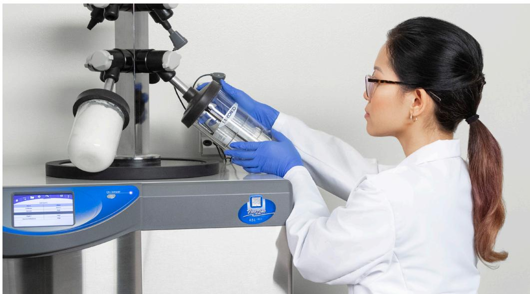
In the manifold method, flasks are individually attached to the ports of a drying chamber.
