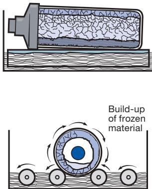
**Figure 6:** Shell freezing can increase the surface area to volume ratio by spreading out the frozen product inside the vessel.
