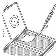
4. Roll blot membrane gently to remove air bubbles.
