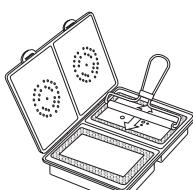
5. Place the spacer (wetting not necessary) on top of the blot membrane and roll again to ensure contact of spacer with blot membrane.
