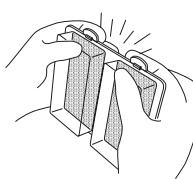
8. Open lid of system and place blot holder in chamber, aligning blot holder tabs with notches of chamber. Close and latch lid.
