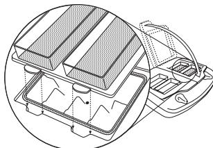
9. Add volume of blocking solution as indicated under **OPTIMIZATION GUIDELINES** on reverse side. Using knobs on the system, apply vacuum until well(s) are completely empty.
