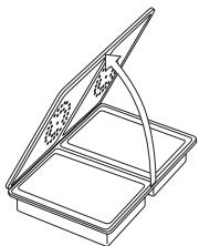
2. Thoroughly wet the white surface of the blot holder with Milli-Q® water.
