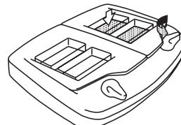
10. Add volume of primary antibody as indicated under **OPTIMIZATION GUIDELINES** on reverse side. Antibody solution must evenly cover **entire** blot holder surface.
