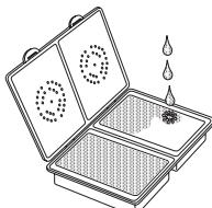
3. Place the pre-wet blot in the center of the blot holder with the protein side down. The blot membrane should not exceed size specified in the User Guide.
